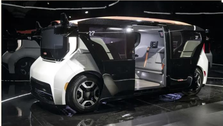
The Cruise Origin is an all-electric vehicle resembling a lounge on wheels with no steering wheel or pedals © Bloomberg
